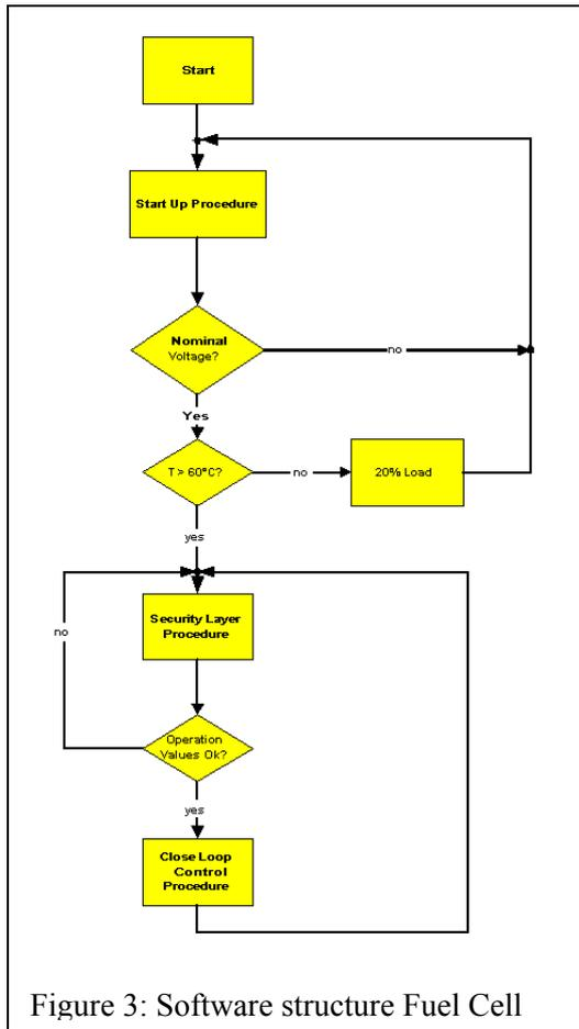
There exist different software tasks: first the Start Up of the FC stack, second the security layer, third the shut down of the stack and last the Closed Loop Control.
