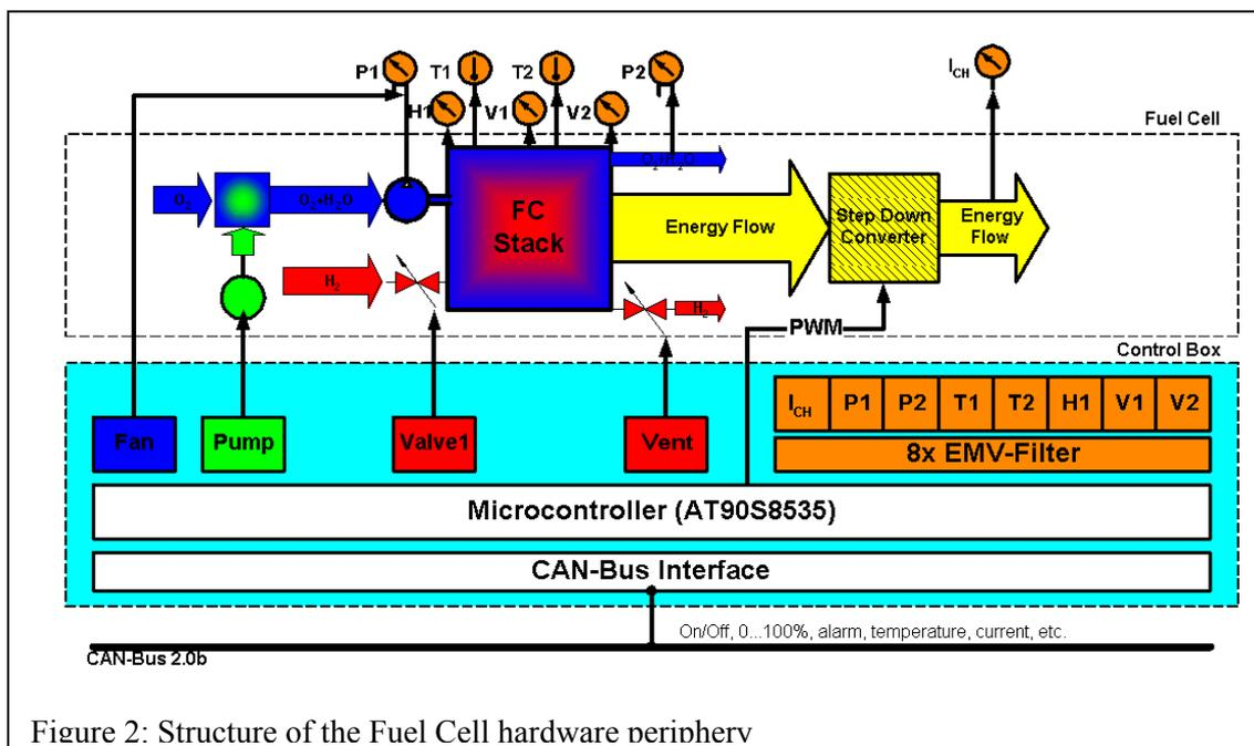
Figure 2: Structure of the Fuel Cell hardware periphery
