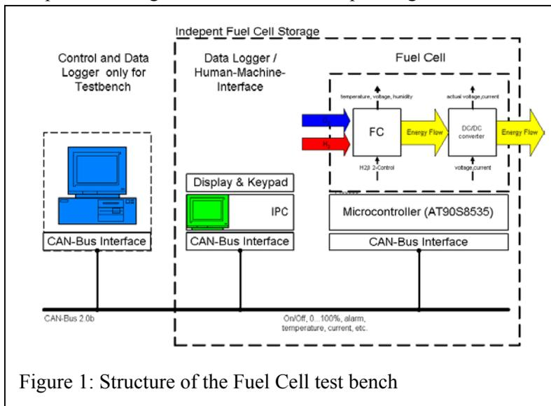
Figure 1: Structure of the Fuel Cell test bench
