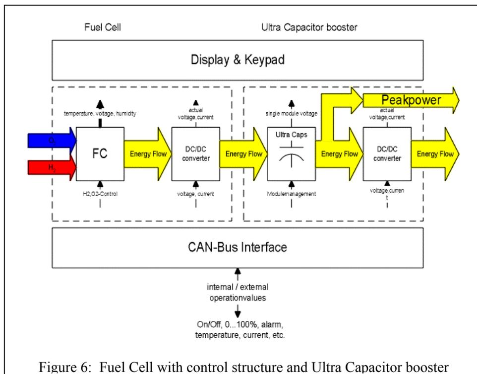
Figure 6: Fuel Cell with control structure and Ultra Capacitor booster
